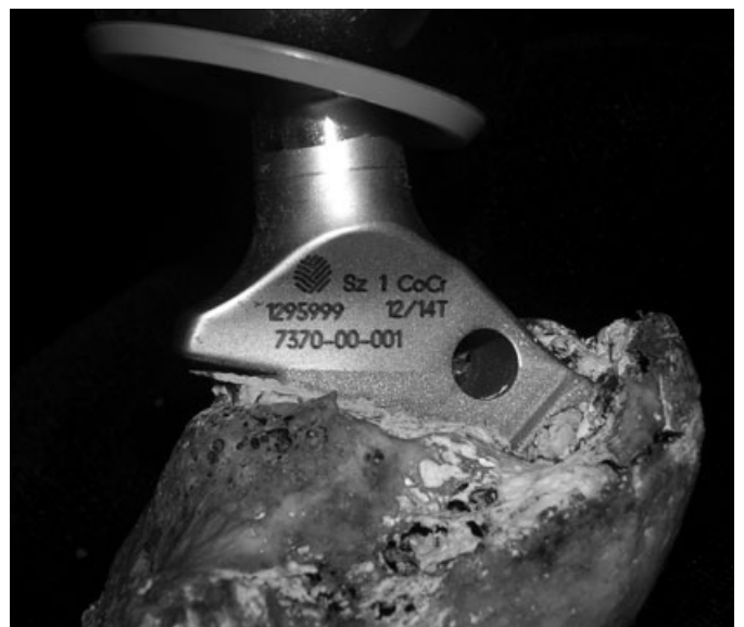
FIG. 6—An example of a femoral implant that clearly indicates the company logo, serial number, part/lot number, and other product information.
