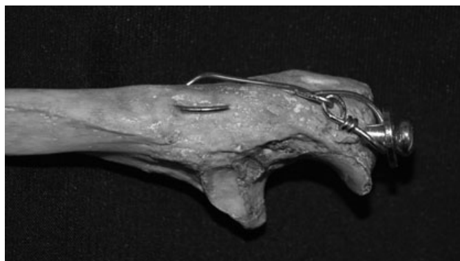
FIG. 1—The screw and washer in this proximal ulna is an example of a common implant to find throughout the skeleton.
